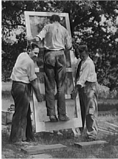
Testing homemade screen door for strength.
